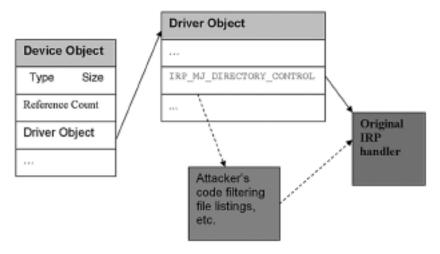
Figure 4. Illustration of hooking a driver's IRP table
