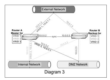
and B, are connected to all three networks, and are also connected to each other via a crossover cable for Firewall-1 state synchronization (discussed below). Under normal conditions, Firewall A will serve as master for the three VRIDs (one on each network), while Firewall B will serve as backup.
